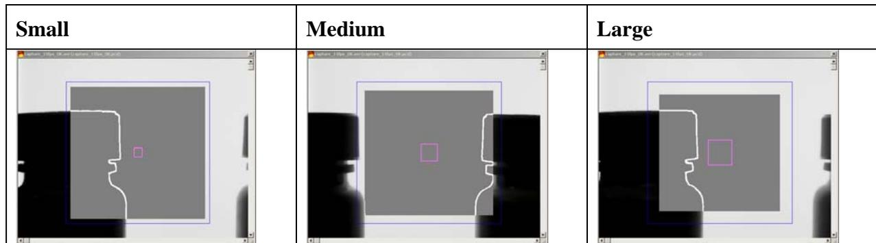
Choose a feature size so the feature fits over a typical defect part of the image. In the above example, we want to detect a slightly loose bottle cap. You can see that the Medium feature size in the center image is correct for the desired inspection – the feature will correctly guide learning so the shape of the small gap between the cap and the bottle can be very accurately judged.
