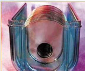
Product: Hard Disks Inspection Objective: Inspect for missing, cross-slotted, or double disks within tray
